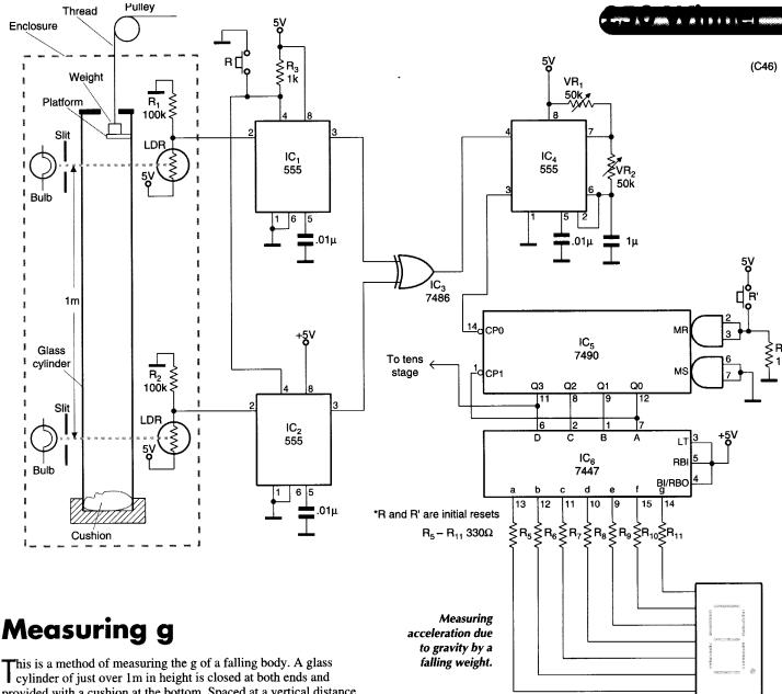
This is a method of incasuring the gold at both ends and cylinder of just over 1m in height is closed at a vertical dist provided with a cushion at the bottom. Spaced at a vertical distance of exactly 1m are bulbs, slits and light-dependent resistors. These detect the passing of the falling body, which is initially kept in place by a removable platform and further retained by a thread when the platform is taken out.
